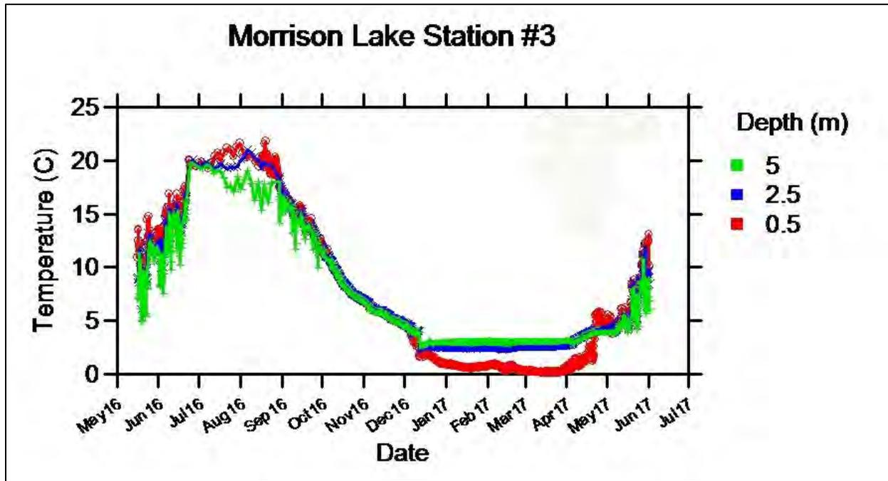
Figure 3-9 Temperature data from Station #3 thermistor chain.
