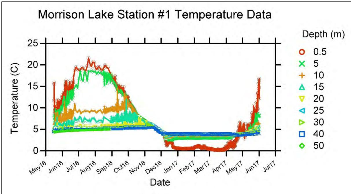
**Figure 3-3 Temperature data from Station #1 thermistor chain.**
