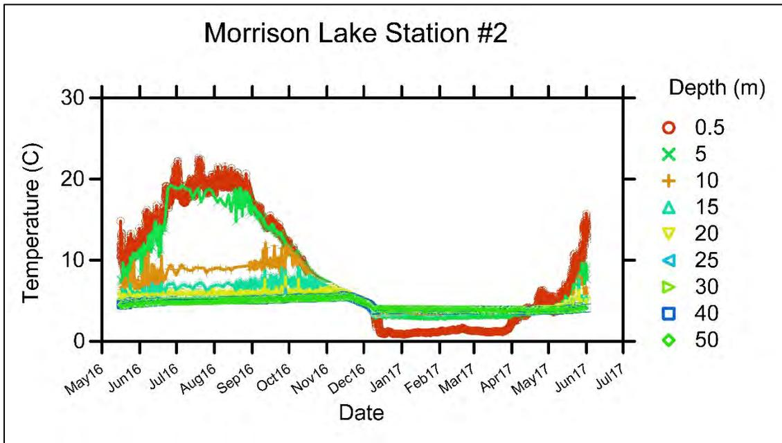
Figure 3-8 Temperature data from Station #2 thermistor chain.
